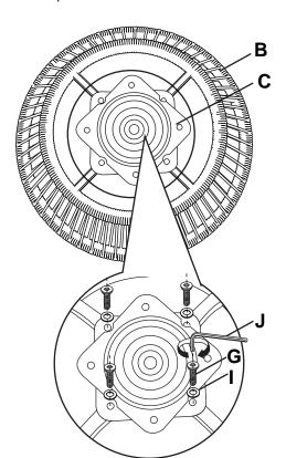
Turn upside down seat top (A) on a protected surface, use Allen key (J) to fix seat base (B) on seat top (A) with bolts (G) and washers (I) as picture.
